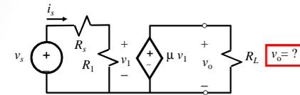
$v_1 = \frac{R_1}{R_1 + R_s} v_s$
