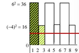
$$V_{rms} = \sqrt{\frac{1}{3} \left( \int_0^2 6^2 dt + \int_2^3 (-4)^2 dt \right)} = \sqrt{\frac{1}{3} (72 + 16)} = \sqrt{\frac{88}{3}} \text{ V}$$
