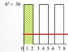
$$V_{rms} = \sqrt{\frac{1}{3} \int_0^2 6^2 dt} = \sqrt{\frac{1}{3} (36t)_0^2} = \sqrt{\frac{72}{3}} \text{ V}$$
