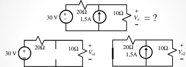
$V_{o1} = \frac{10}{10+20} \times 30 = 10 \text{ V}$
