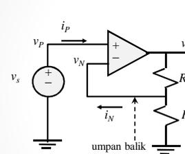
$$v_N = \frac{R_2}{R_1 + R_2} v_o$$
